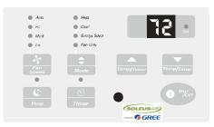
Note: Press this button, Sleep On and Sleep Off can be selected. When the unit is on, Sleep Off is defaulted. After the unit is shut off, the Sleep function is canceled. If the unit is in Cool or Energy Saver Modes, and the Sleep Mode is set, the SET TEMP. will increase 2\*F in 1 hour and 4\*F in 2 hours. If the unit is in Heat Mode, and Sleep Mode is set, the SET TEMP. would decrease 2\*F in 1 hour and 4\*F in 2 hours.
